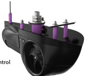
By adding the Hydropod low drag cover, the new SX models can be mounted under the hull in the water flow for low- and mid-speed vessels. The optimal design adds minimal drag and will in most installations not be noticeable. For a typical sail boat cruising at 7,5 knots, the added drag is **less than 3kg.** The in-flow configuration is perfect for boats where it is difficult to fit a tunnel thruster or for example as stern thruster for cruising sailboats.
