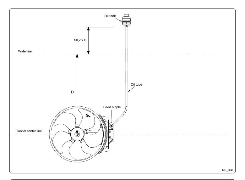
Oil Tank Installation MC\_0023
