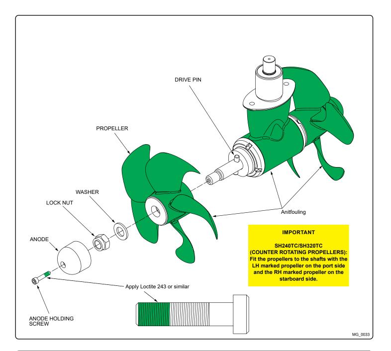
Propeller Installation MC\_0018
