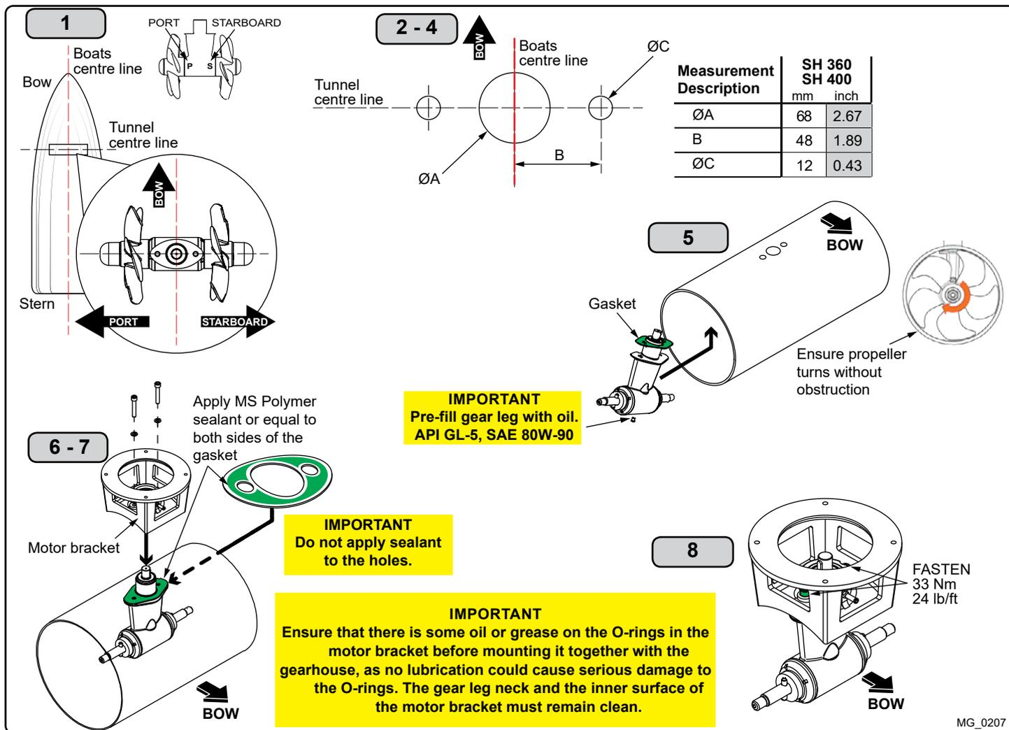
**EN Gear Leg & Motor Bracket Installation MC\_0001**
