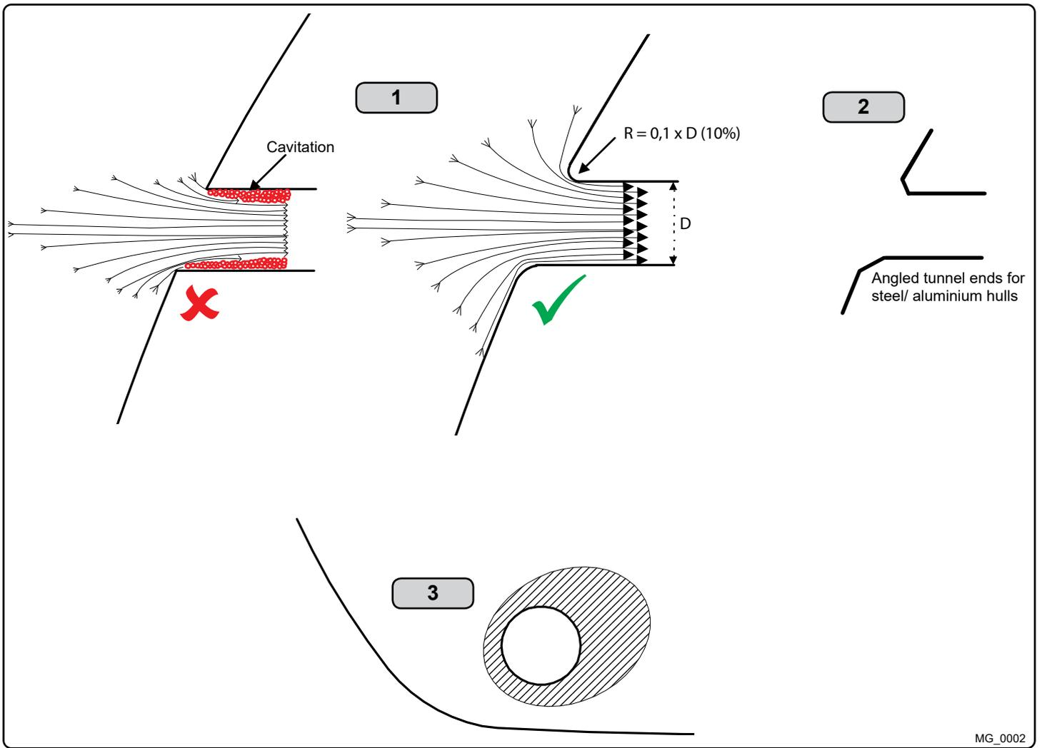
**Rounded tunnel ends will maximise thrust and minimise noise and cavitation.**
