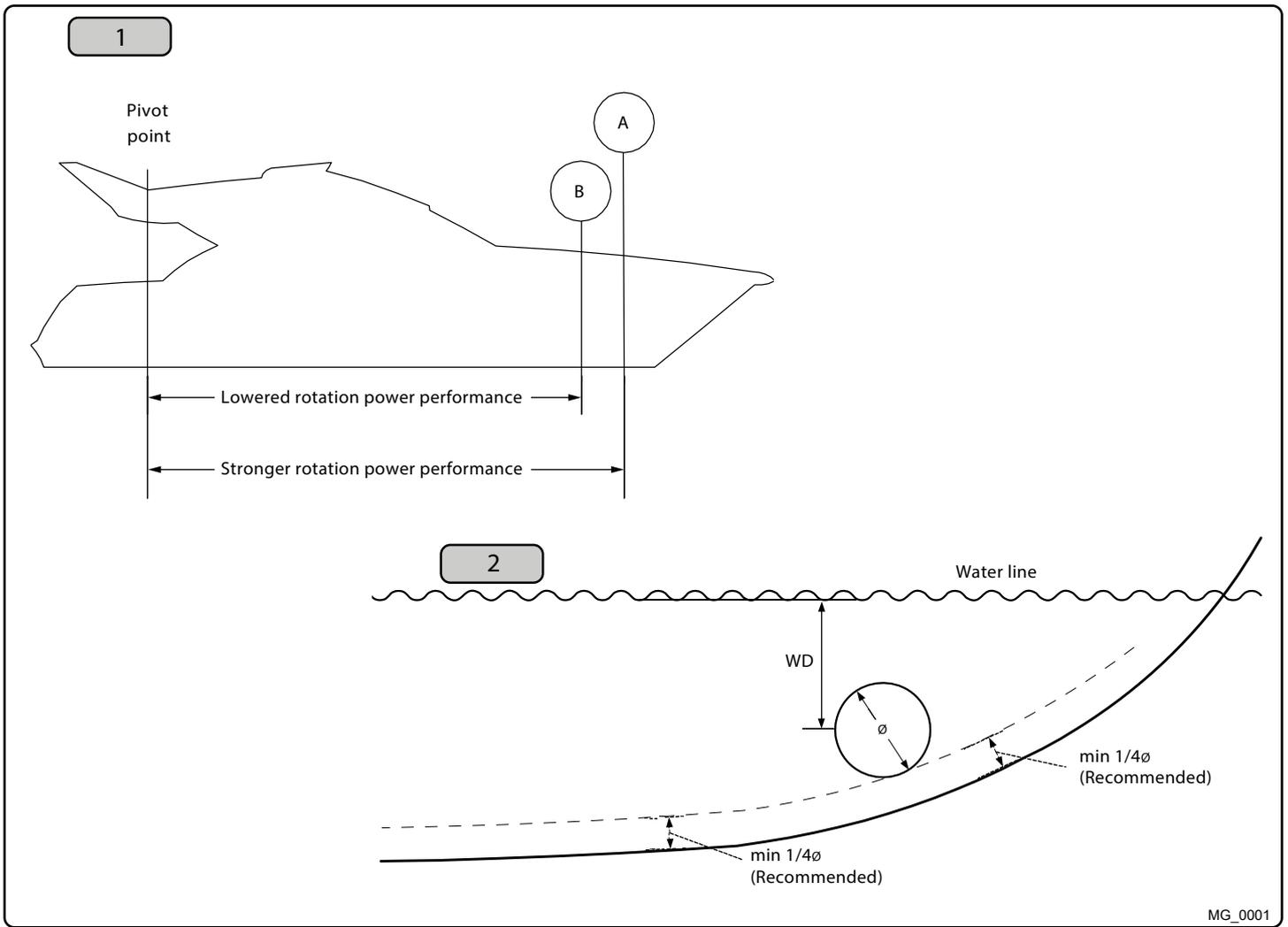
**EN** **Positioning of the tunnel / thruster** **MC\_0003**
